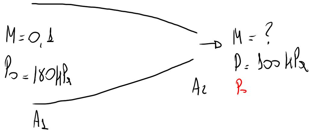
$$h_{01} = h_1 + \frac{V_1^2}{2} = h_2 + \frac{V_2^2}{2} = h_{02}$$
